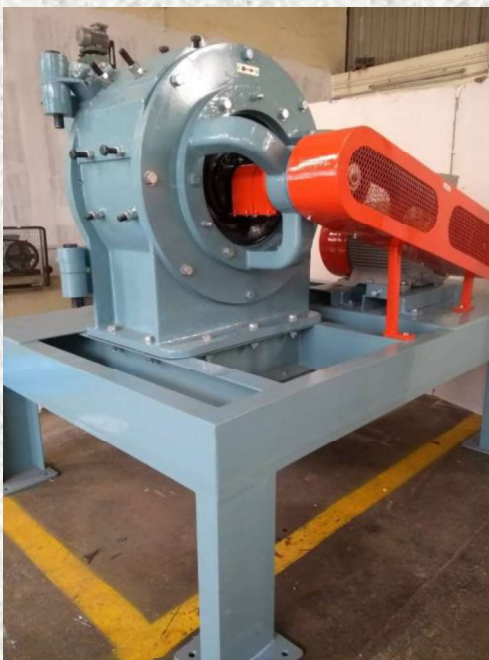
Rotor crusher mill with hot gas system for drying and pneumatic transport of ground product
